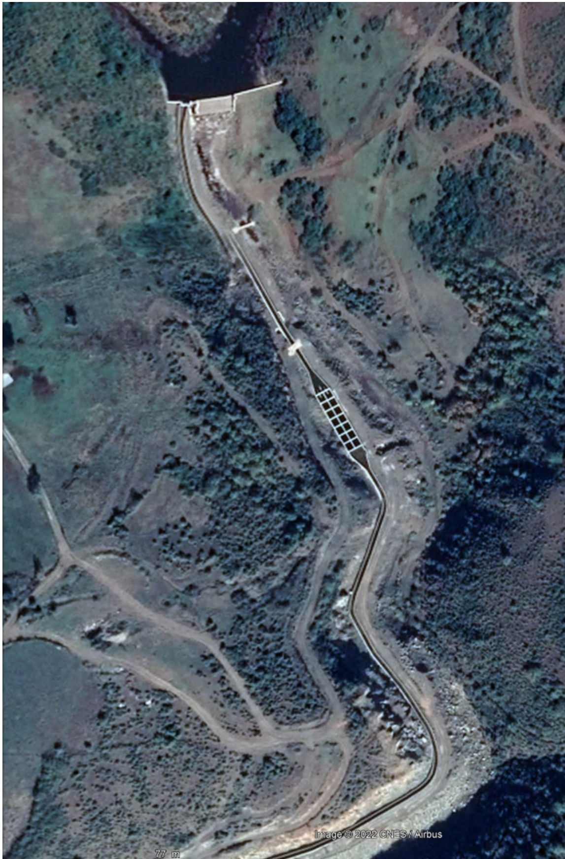
Figure 33: HPP on Skatina River: The “new concrete river” with total water abstraction (GE 2022).
