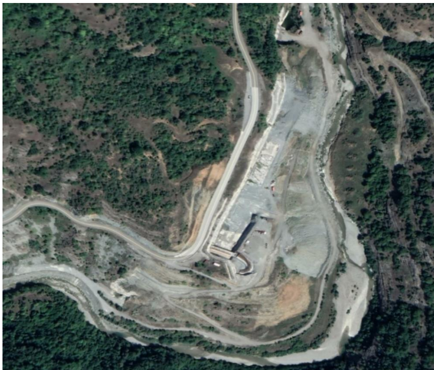
Figure 40: On Aliakmonas, the largest river north of the Aoo catchment, hydropower construction has already begun and SHPs are planned to be developed in the upstream of this sparsely populated area. While this picture features a bigger SHP with some 7 MW, many of the 0.1-1 MW SHPs look similar to those in Albania, with long pipes diverting the river water, causing very little discharges in the former river bed (GE 2022).
