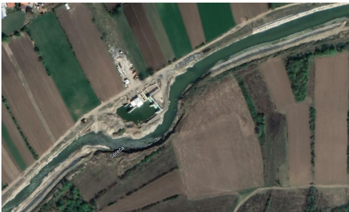
Figure 15: Spreča SHP, illustrating the typical construction site for a run-of-the-river plant including the regulation and reinforcement of the impoundment stretch upstream and the erosive downstream reach (GE 2022).
