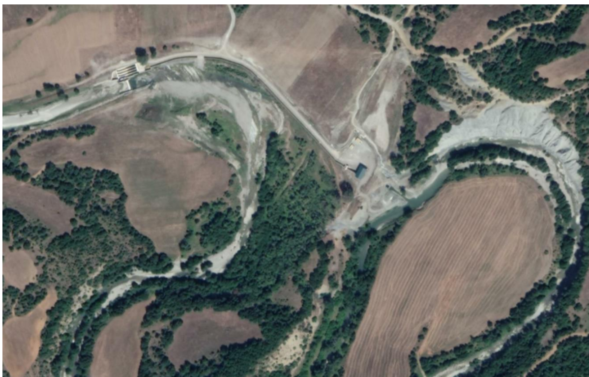
Figure 41: SHP on Grevena River whose tailrace canal cuts off the entire valley meander (GE 2022).
